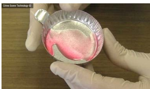
Lumicyano™ in the liquid state before fuming. © Crime Scene Technology. This image is available from the CNRS photo library, phototheque@cnrs-bellevue.fr
