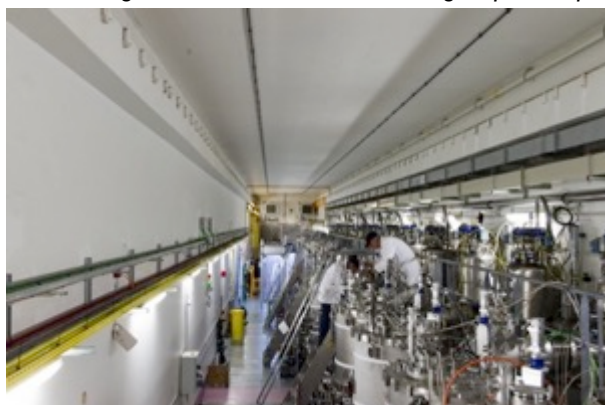
The Spiral2 Linac (LINear ACcelerator) with its superconducting cryomodules enclosing the accelerator cavities. © Philippe Stroppa/CEA/CNRS
