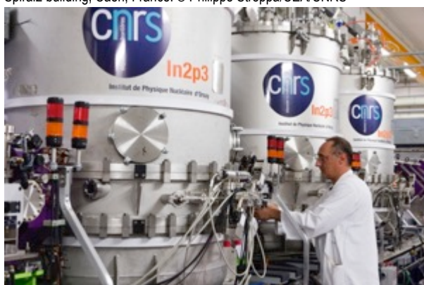
Superconducting cryomodules enclosing the accelerator cavities of the Spiral2 Linac (LINear ACcelerator). © Philippe Stroppa/CEA/CNRS
