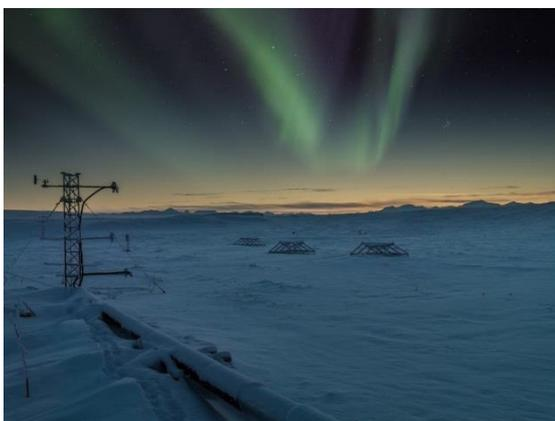
**Installation for mercury flux measurements at Toolik Field Station**
