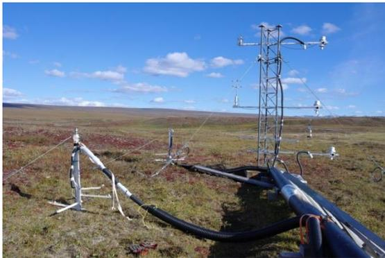
**Flux tower measuring mercury exchange in the tundra at Toolik Field Station in Alaska**
