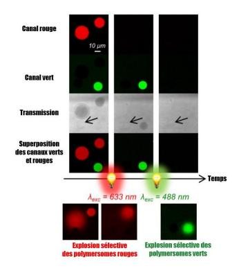
Confocal microscope observations of three types of vesicles. In red, methylene blue-loaded vesicles; in green, calcein-loaded vesicles. Sucrose-loaded vesicles are indicated by an arrow. Laser irradiation of 633 nm then 488 nm ruptures the red and green vesicles in succession. The other vesicle remains intact. © Peyret et al. 2016.
