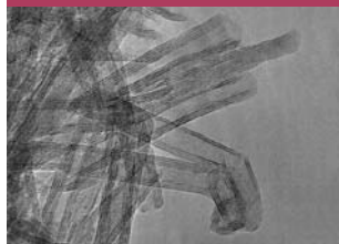
Image of titanium oxide nanotubes using very high resolution electronic microscopy.
