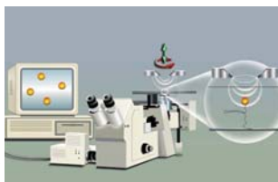
Magnetic microballs, anchored by a DNA molecule to the surface of a capillary tube, are observed using an inverted microscope.
