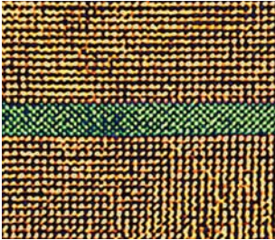
Cross-sectional view of a magnetorestrictive tunnel junction using high-resolution electronic microscopy.
