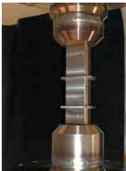
Lisor T 91 sample tube. This device, designed for studying various structural materials subjected to radiation, in contact with liquid metals and under mechanical constraint has been developed within the framework of the Gédéon Research Grouping (waste management through new options from the PACE program).
