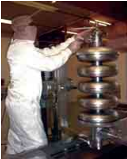
© IPN Orsay. Component of a modern accelerator: superconductor cavity made of niobium. The importance of the cleanliness of the surface explains why the work is being carried out in a clean room.
