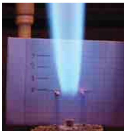
Stabilization of a flame using plasma.
