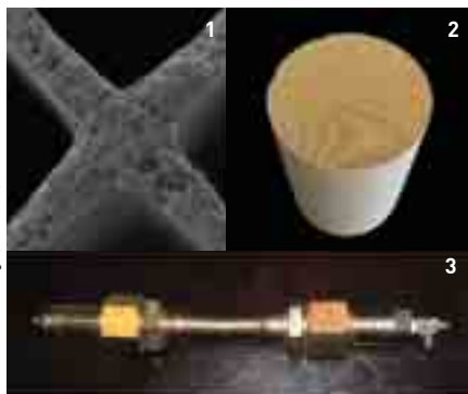
View of a catalytic process of hydrogen production on a structured reactor, from the nanoscopic scale (monolith crosspiece in honeycomb covered with its catalytic layer – figure 1) to the laboratory reactor (equivalent to a power of 1 kW – figure 3), via the overall structure of the monolith (figure 2).
