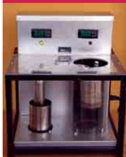
Tested on this cycling test bank, the solid-gas thermochemical system developed by CNRS makes it possible to generate cold using heat, rather than electricity. This process has numerous benefits: complete autonomy, reduced footprint and total absence of sound or vibration.
