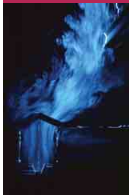
Visualization of air movement within buildings (in the vicinity of an air vent on the photo) contributes to understanding turbulence and provides better ways to control heat transfer.
