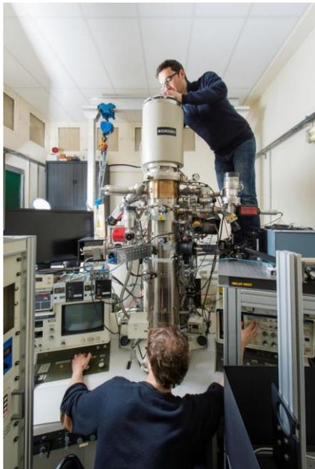
**CEMES researchers handling the prototype of the ultrafast coherent TEM microscope.**
