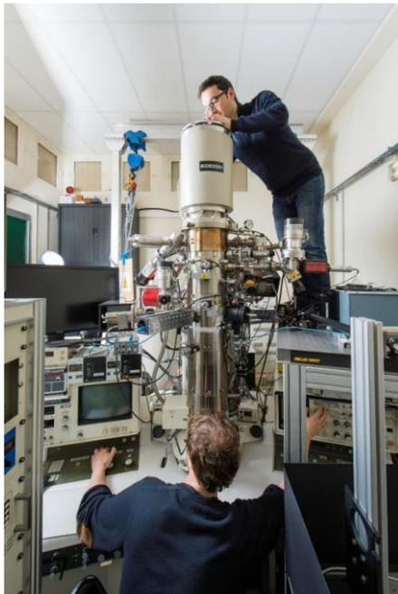
**CEMES researchers handling the prototype of the ultrafast coherent FemtoTEM microscope.**
