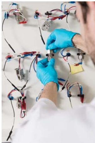
Plugging a cell for basic research on sodium-ion (Na-ion) battery materials. Its performance will thus be electro-chemically tested.
