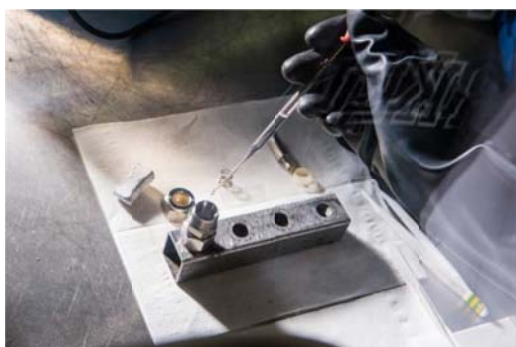
Assembling a cell to test sodium-ion (Na-ion), battery materials in a glove box.
