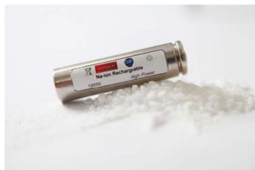
Standard "18650" sodium-ion (Na-ion) battery placed on a heap of salt (NaCl). This is the first-ever sodium battery in this format.
