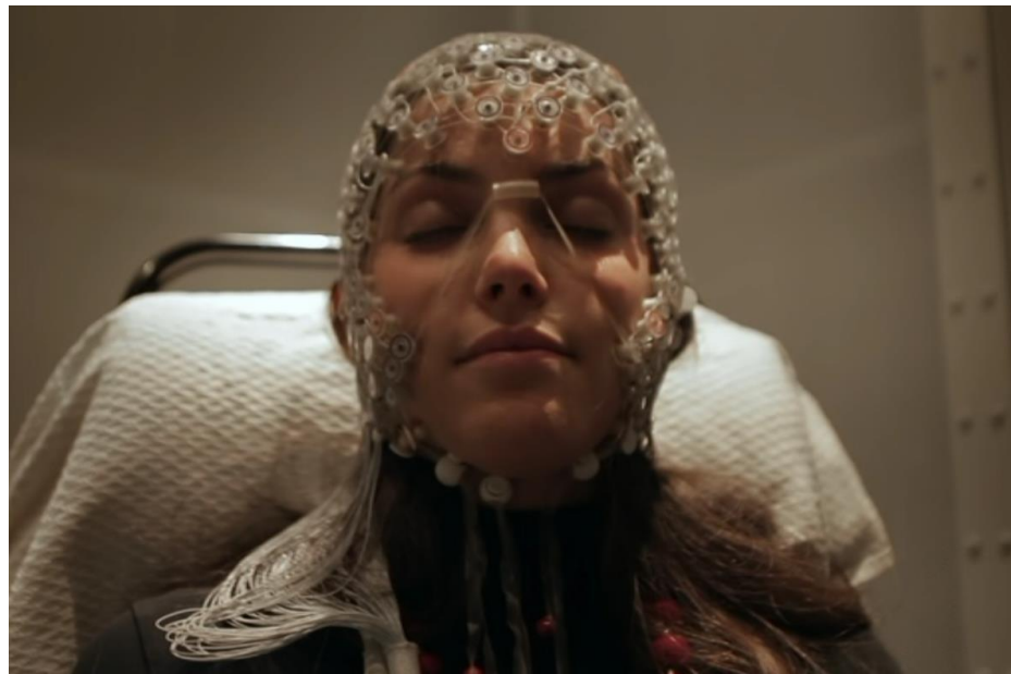
Participant of a sleep experiment equipped with an electroencephalogram. The electroencephalogram records brain's electrical activity and allows to determine in real time whether a person is awake or asleep. Response handles placed in participants' hands allowed them to categorise the sounds presented during the experiment © Scientifilms - Déchiffrer la conscience, voyage dans l'étoffe de nos pensées.
