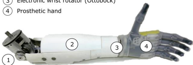
The arm prosthesis prototype used for the experiments, composed of a motorized elbow (1), an electronic wrist rotator (3) and a polydigital hand, the Touch Bionics Robolimb (4).
