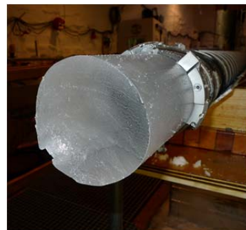
Once the corer is at the surface it is placed horizontally to allow the ice core to be removed. The ice core has a diameter of 10.2 cm and a length of 3.5 meters. © Sepp Kipfstuhl, Alfred Wegener Institute, Bremerhaven, Germany
