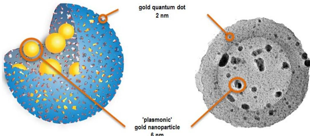
Diagram and electronic microscopy image of a "quantum rattle": a porous silica shell (in blue in the diagram) is filled with gold dots, all on a nanometric scale.
