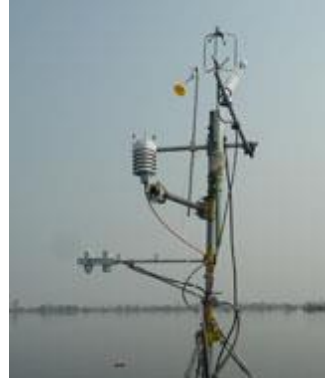
A micrometeorological station that continuously measures methane fluxes.
