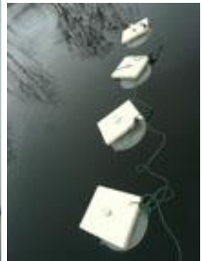
The submerged funnels trap methane bubbles that rise up from the bottom of the reservoir.
