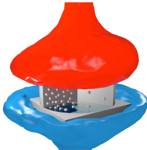
*Artist's impression of the electronic synapse: the particles represent electrons circulating through oxide, by analogy with neurotransmitters in biological synapses. The flow of electrons depends on the oxide's ferroelectric domain structure, which is controlled by electric voltage pulses. © Sören Boyn / CNRS/Thales physics joint research unit.*
