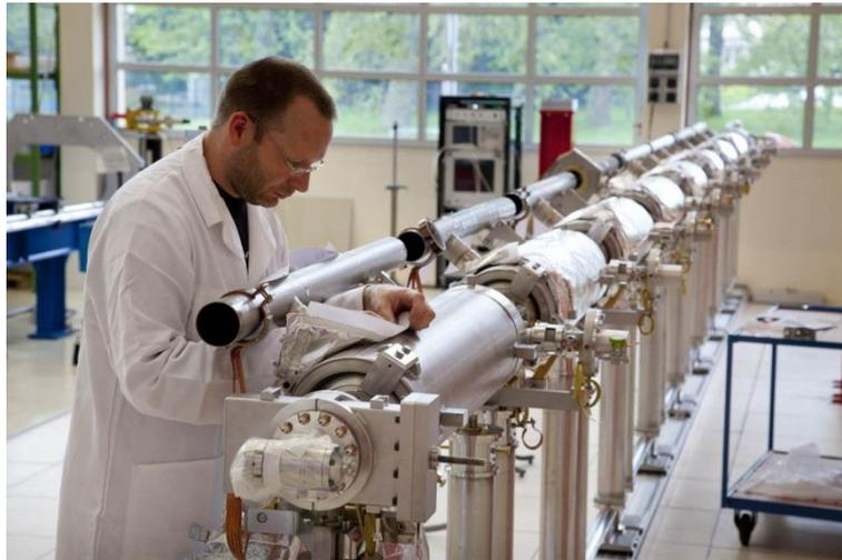
Assembly of cryogenic helium distribution system for series of cavities along XFEL © Dumas / CEA
