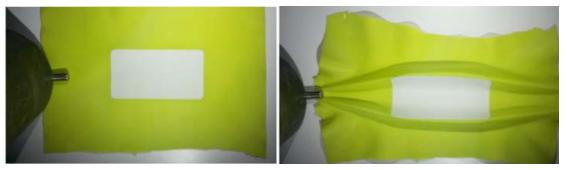
Modeling of the fold formation mechanism. A sheet of rubber on which a (stiffer) paper label is stuck buckles along the boundary between the stiff zone and the soft zone when it is stretched. This reproduces the formation of folds along the boundaries between cellular domains.
