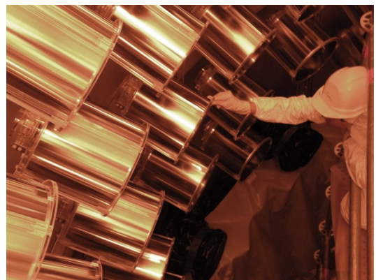
Photomultipliers on the inside of the tank.
