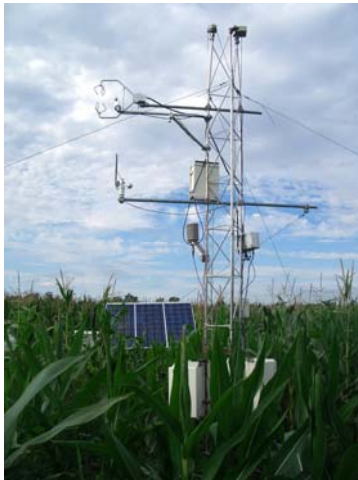
Flux tower installed in the middle of a maize crop, equipped with analyzers and sensors for measuring fluxes and meteorological variables. © Eric Ceschia
