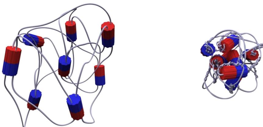
Left: Schematic representation of a polymer gel whose chains are cross-linked using rotating molecular motors (the red and blue parts of the motor can turn relative to each other when provided with energy).
